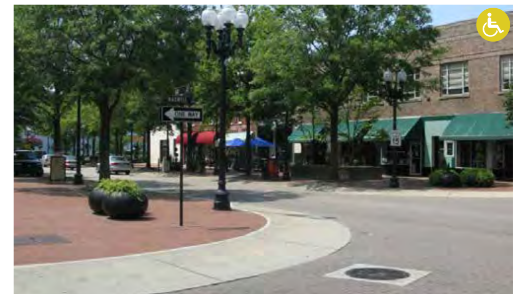
Photo Source: www.nacto.org - Raised Table Intersection with feature paving. Source: National Association of City Transportation Officials. North America
